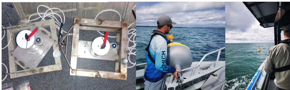
Figure 8. Deploying continuously logging PAR equipment in Hervey Bay May 2022.
