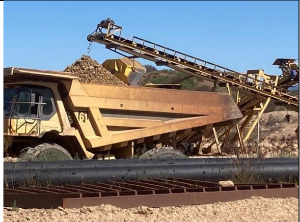
Figure 15: Oversize from Screen conveyed into Truck
