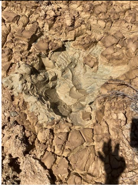
Figure 19: PL2 Wet Tails showing crusting
