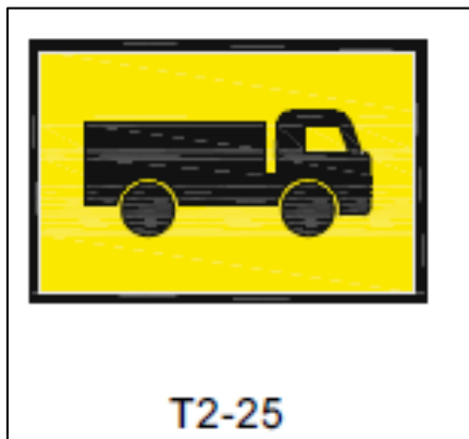
Figure 7.3 Trucks crossing or entering (T2-25) warning sign Australian Standard AS1742.2
